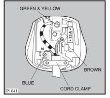
The wire coloured green and yellow must be connected to the terminal marked with the letter «E» or by the earth symbol  $\stackrel{-}{=}$  or coloured green and yellow.
