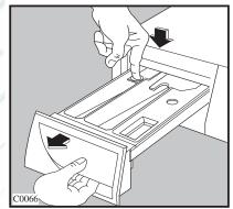
To aid cleaning, the top part of the additive compartment should be removed. Clean all parts with water.
