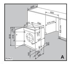
When installing the appliance into the kitchen furniture ensure, if possible, the hoses are placed in either of the two recesses on the back of the appliance. This will help to prevent the hoses from becoming kinked or trapped.
