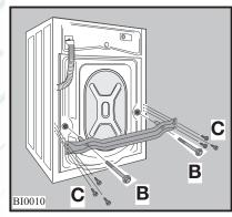
5. Remove the bracket **D** and refit the six smaller bolts **C**.
