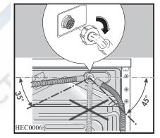
3. Set the hose correctly by loosening the ring nut.
