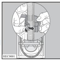
3. With the supplied spanner unscrew and remove the central rear bolt **A**. Slide out the relevant plastic spacer.
