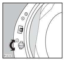
To disable this device and restore the possibility of closing the door, rotate the button anti-clockwise until the groove is vertical.
